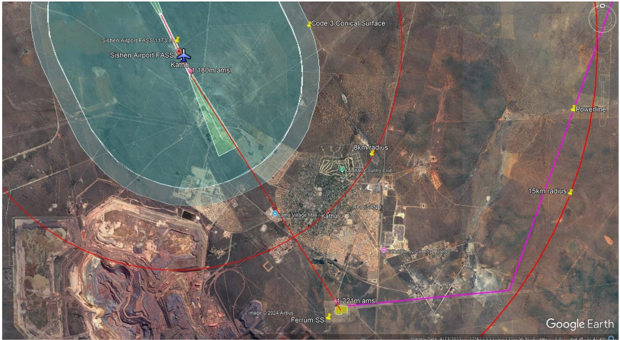
Figure 4: Ferrum SS relative to ICAO Obstacle Limitation Surfaces near Kathu (FASS)
